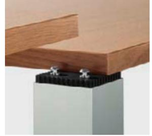
The method for connecting the rigid table tops to the table legs is ingenious: open the bayonet lock, lift the table top up, move the table leg, add the next table top and apply the bayonet lock again.
